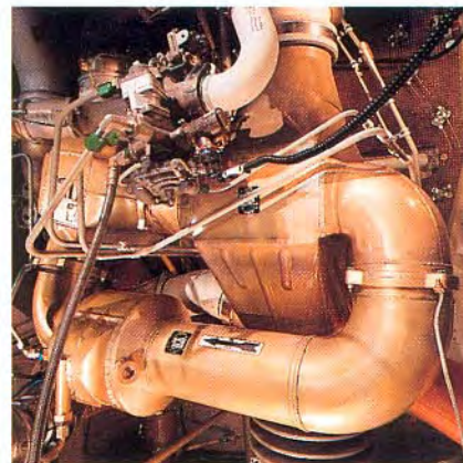
Air conditioning pack
