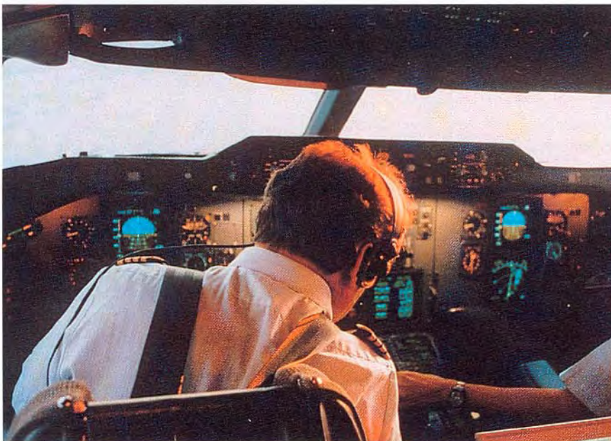
A310 cockpit with left pilot's (CM1) PGS in view at extreme left of glareshield.
